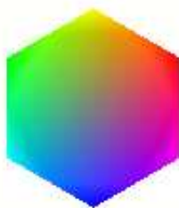
Fig. 15.3: The colour hexagon used for analyzing the colour content of the PCA and ICA features. The hexagon is the projection of the RGB cube onto a plane orthogonal to the luminance ( R + G + B ) vector. Thus achromatic RGB triplets map to the center of the hexagon while highly saturated ones are projected close to the edges.
